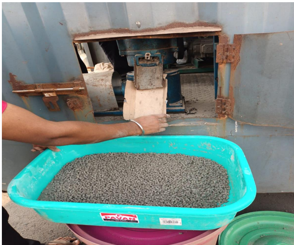
Fig 3: Farm-made pelleted feed preparation using Mobile Feed Mill
